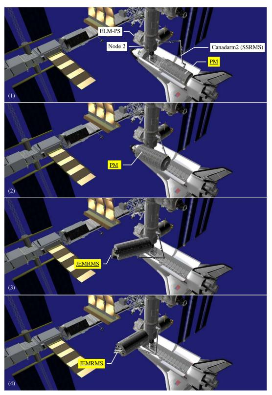
Figure 5.2.2-3 Procedures for attaching PM to ISS
