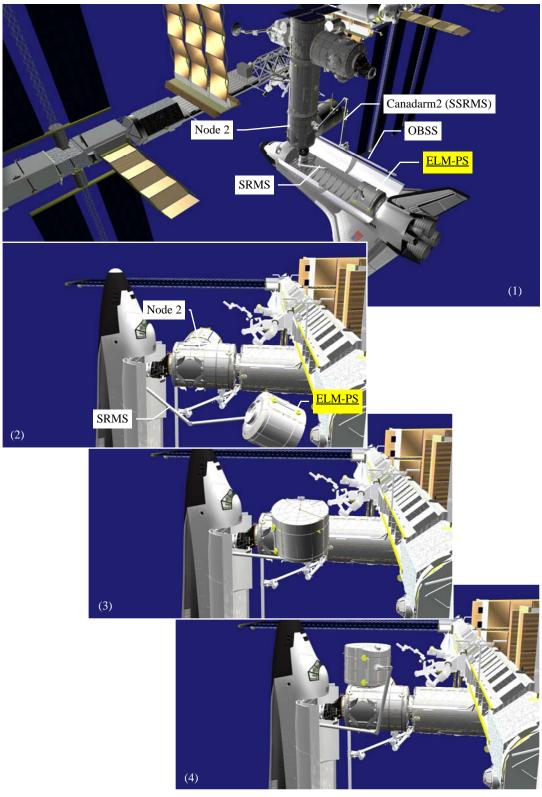
Figure 5.2.1-3 Procedures for connecting ELM-PS to ISS
