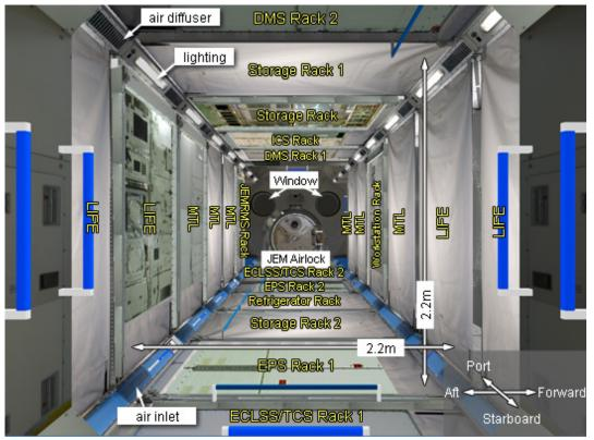
DMS: Data Management System EPS: Electric Power System ECLSS: Environmental Control and Life Support System TCS: Thermal Control System LIFE: Life Science Payload Rack MTL: Material Science Payload Rack
