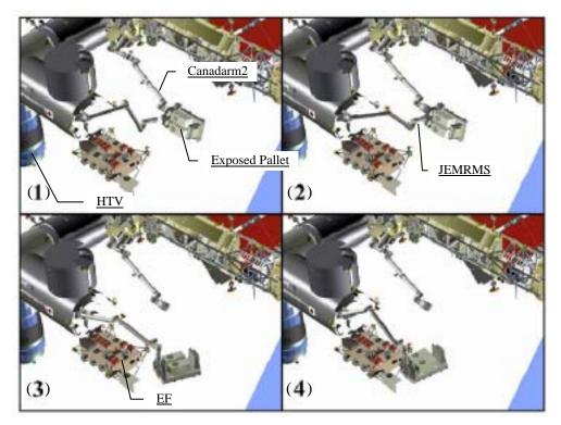
Figure 7.2.4-2 Image of EP attached to EF
