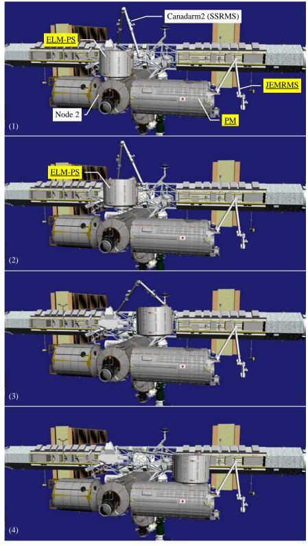
Figure 5.2.2-4 Procedures for relocating ELM-PS (space shuttle is not included)
