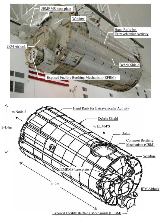
Figure 4.1.2-1 shows an external view and structure of the PM.
