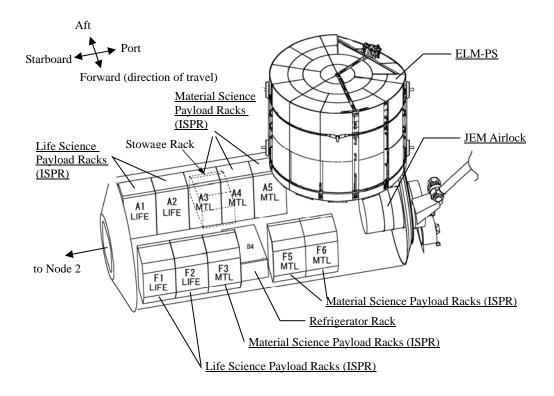
Figure 4.1.2-4 Experiment racks (ISPRs) inside PM
