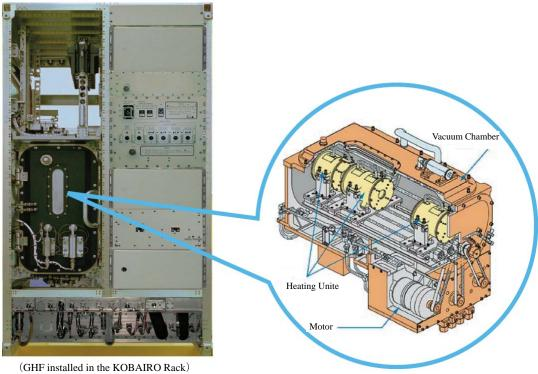
GHF Material Processing Unit (Furnace)
