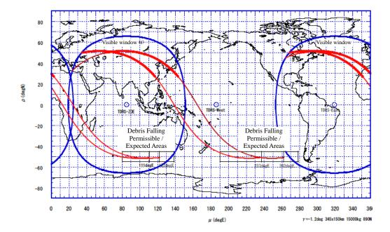
Figure 7.2.5-2 HTV Debris Falling Permissible (Allowed or Expected) Areas and HTV's Orbit (Red lines)
