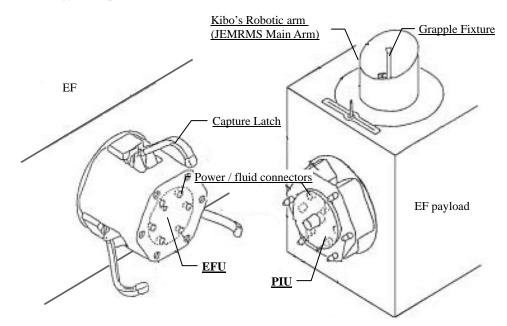
Figure 4.3.3-2 EEU (EFU and PIU) Structures
