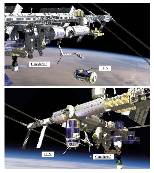
Figure 7.2.3-2 Images of HTV approaching the ISS (above) and HTV Berthing to the ISS (below)
