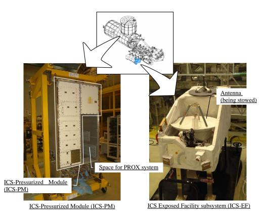
PROX (Proximity Communication System) is a communication system which will be used for a rendezvous operation of the H-II Transfer Vehicle (HTV)
