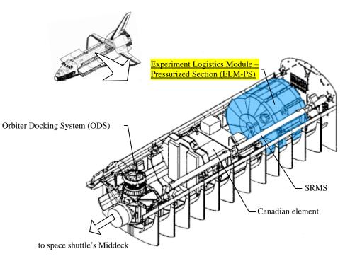
Figure 5.2.1-2 Cargo bay layout during launch of 1J/A Flight (Image)
