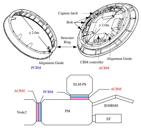
Figure 4.1.3-1 Common Berthing Mechanism (CBM)
