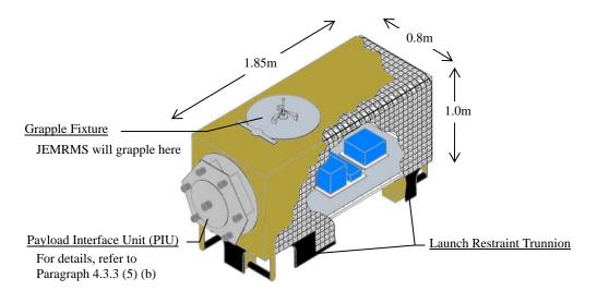
Figure 4.3.1-2 Standard EF Payload
