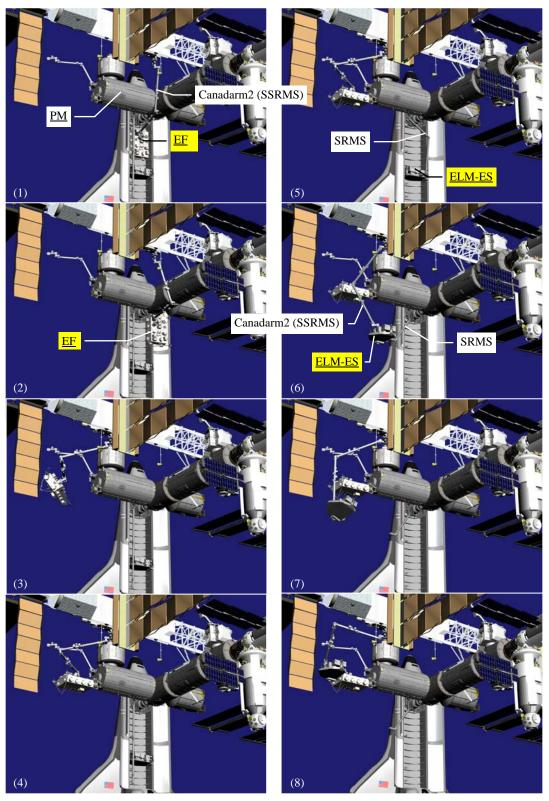
Figure 5.2.3-3 Procedures for connecting EF and ELM-ES to ISS
