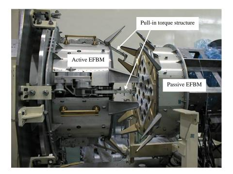
Figure 4.3.3-1 Exposed Facility Berthing Mechanism (EFBM)
