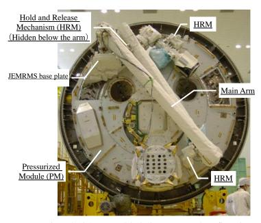
Figure 4.5.3-1 JEMRMS locked to PM (Launch configuration)
