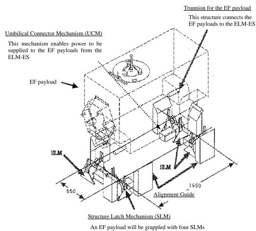
Figure 4.4.3-1 Payload Attachment Mechanism (PAM)
