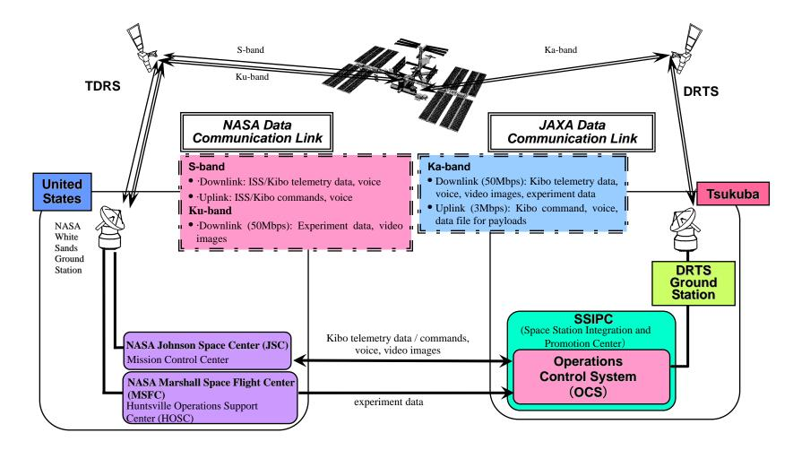
Figure 5.3-3 Conceptual Diagram of orbital/ground communication interfaces for Kibo Operations
