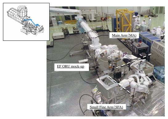
Figure 2.1.5-1 JEM Remote Manipulator System (JEMRMS) -Combination Operation Test
