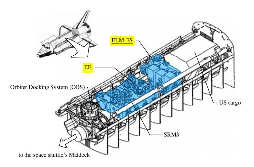
Figure 5.2.3-2 2J/A Cargo bay layout during launch of 2J/A Flight (Image)
