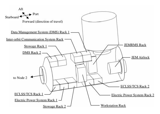
Figure 4.1.2-3 JEM System Racks inside PM
