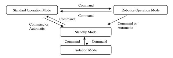
Figure 3.2-1 Kibo Operation Mode Transitions
