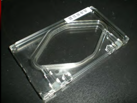
Cell Culture Dish for space (Disposal Culture Chamber(DCC))
