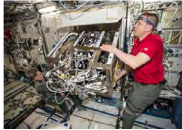
Astronaut install sample holder to ELF.
