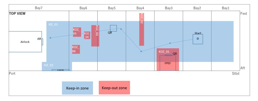
Figure 3.7-1 KIZ and KOZ of the Final Round (Top View)
