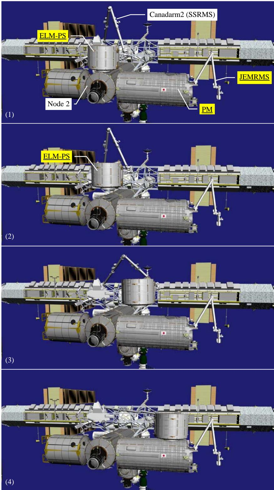
Figure 5.2.2-4 Procedures for relocating ELM-PS (space shuttle is not included)
