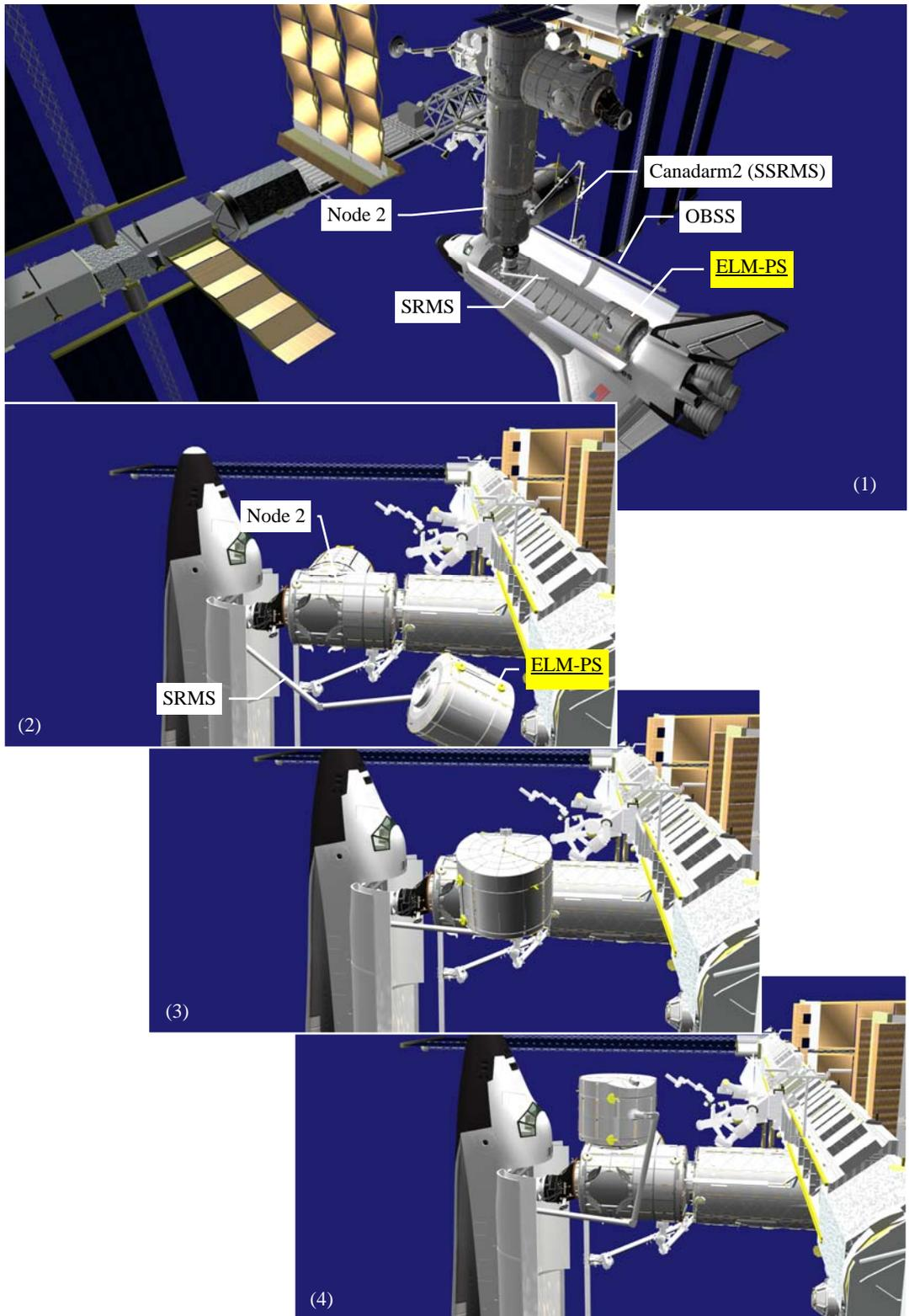
Figure 5.2.1-3 Procedures for connecting ELM-PS to ISS
