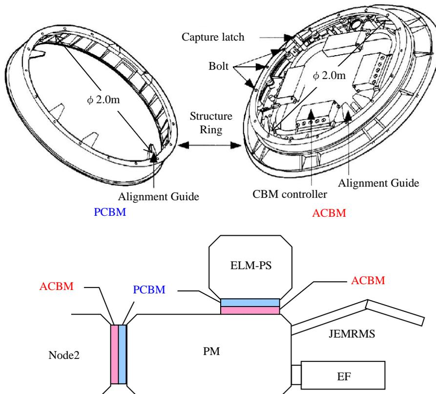
Figure 4.1.3-1 Common Berthing Mechanism (CBM)
