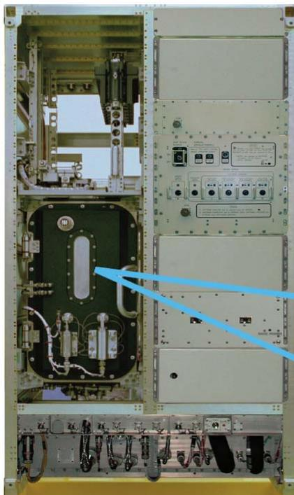
(GHF installed in the KOBAIRO Rack)
