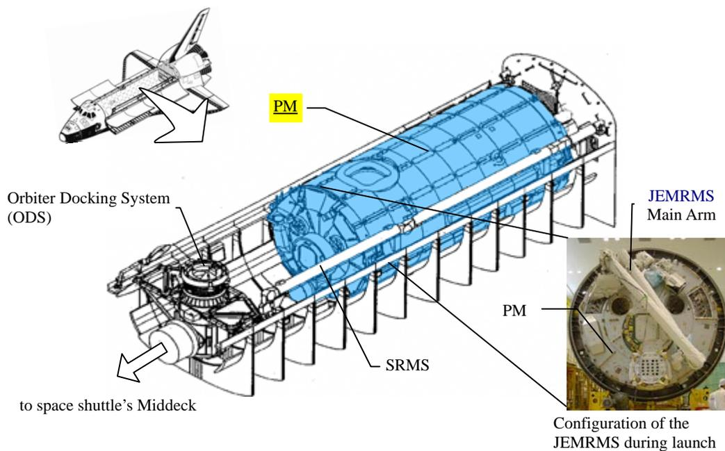
Figure 5.2.2-2 Cargo bay layout during launch of 1J Flight (Image)
