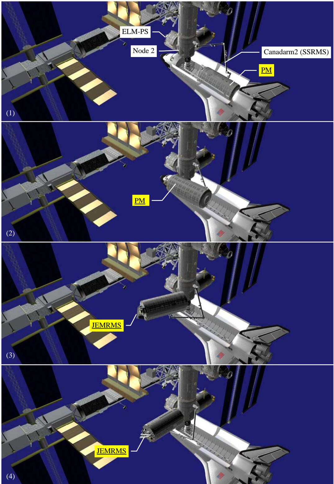
Figure 5.2.2-3 Procedures for attaching PM to ISS
