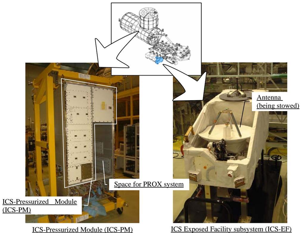
PROX (Proximity Communication System) is a communication system which will be used for a rendezvous operation of the H-II Transfer Vehicle (HTV)
