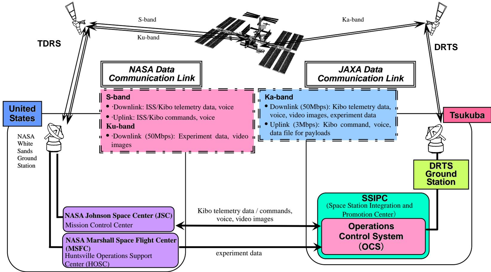
Figure 5.3-3 Conceptual Diagram of orbital/ground communication interfaces for Kibo Operations
