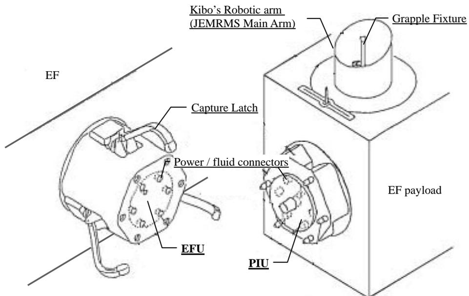
Figure 4.3.3-2 EEU (EFU and PIU) Structures
