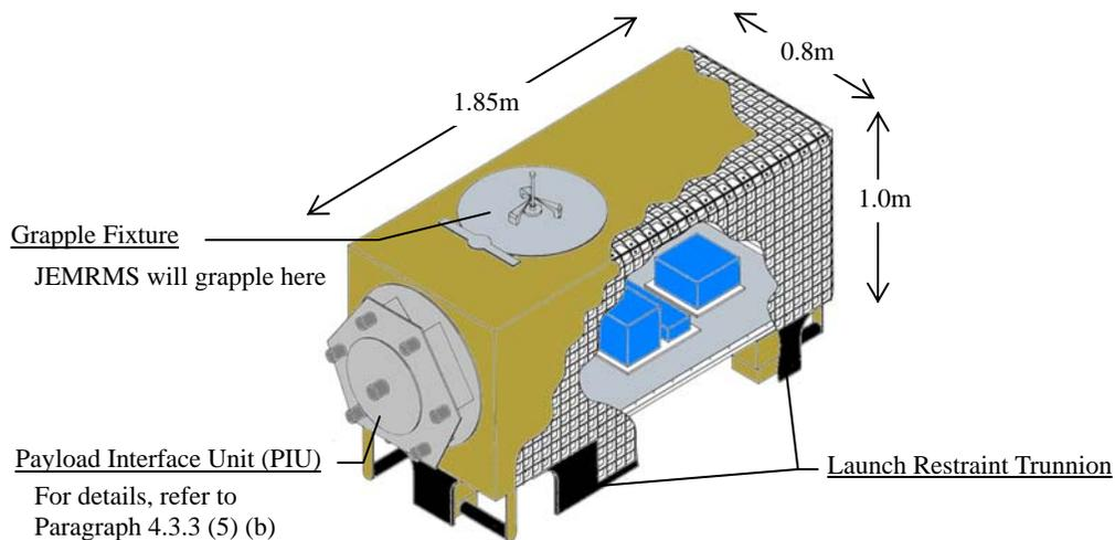
Figure 4.3.1-2 Standard EF Payload
