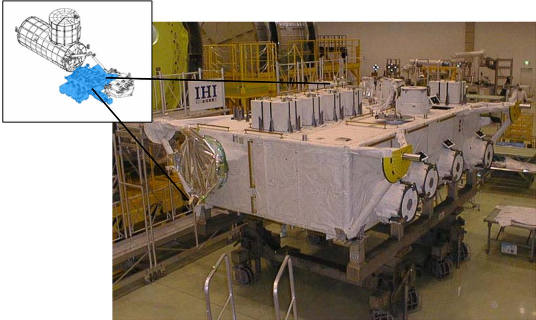
Figure 2.1.3-1 Exposed Facility (EF)
