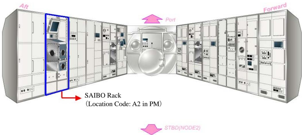
Figure 6.3.1-2 Location of SAIBO Rack in Pressurized Module (PM)
