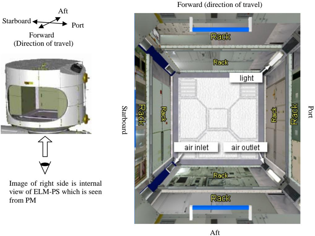
Image of right side is internal view of ELM-PS which is seen from PM
