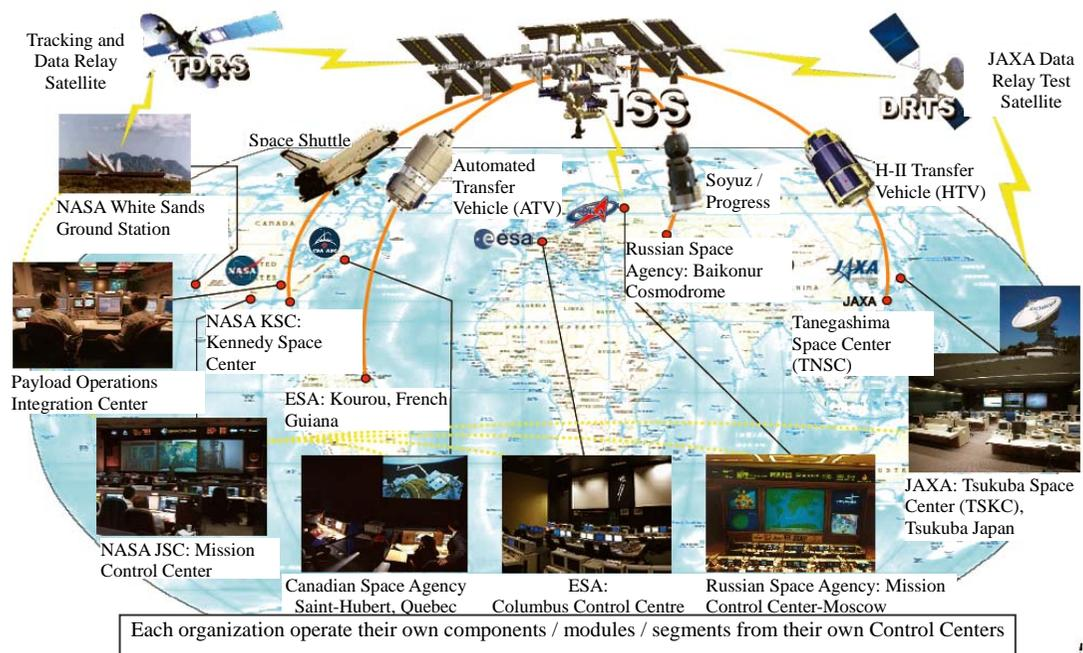
Figure 5.3-1 ISS Operations Conceptual Diagram
