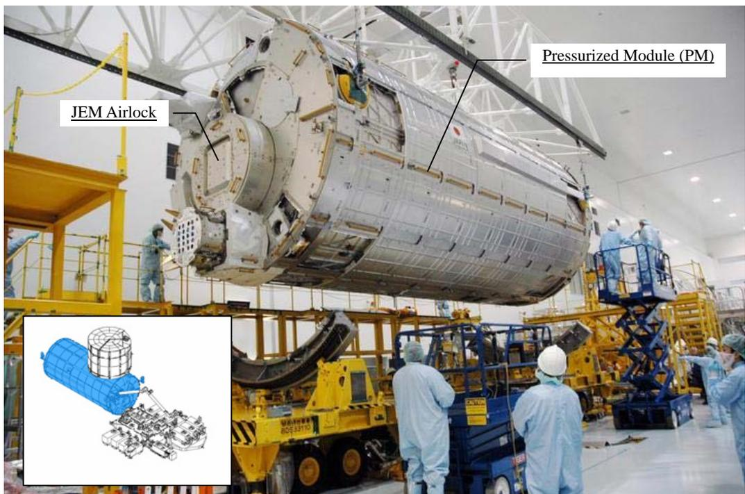
Figure 2.1.1-1 Pressurized Module (PM)
