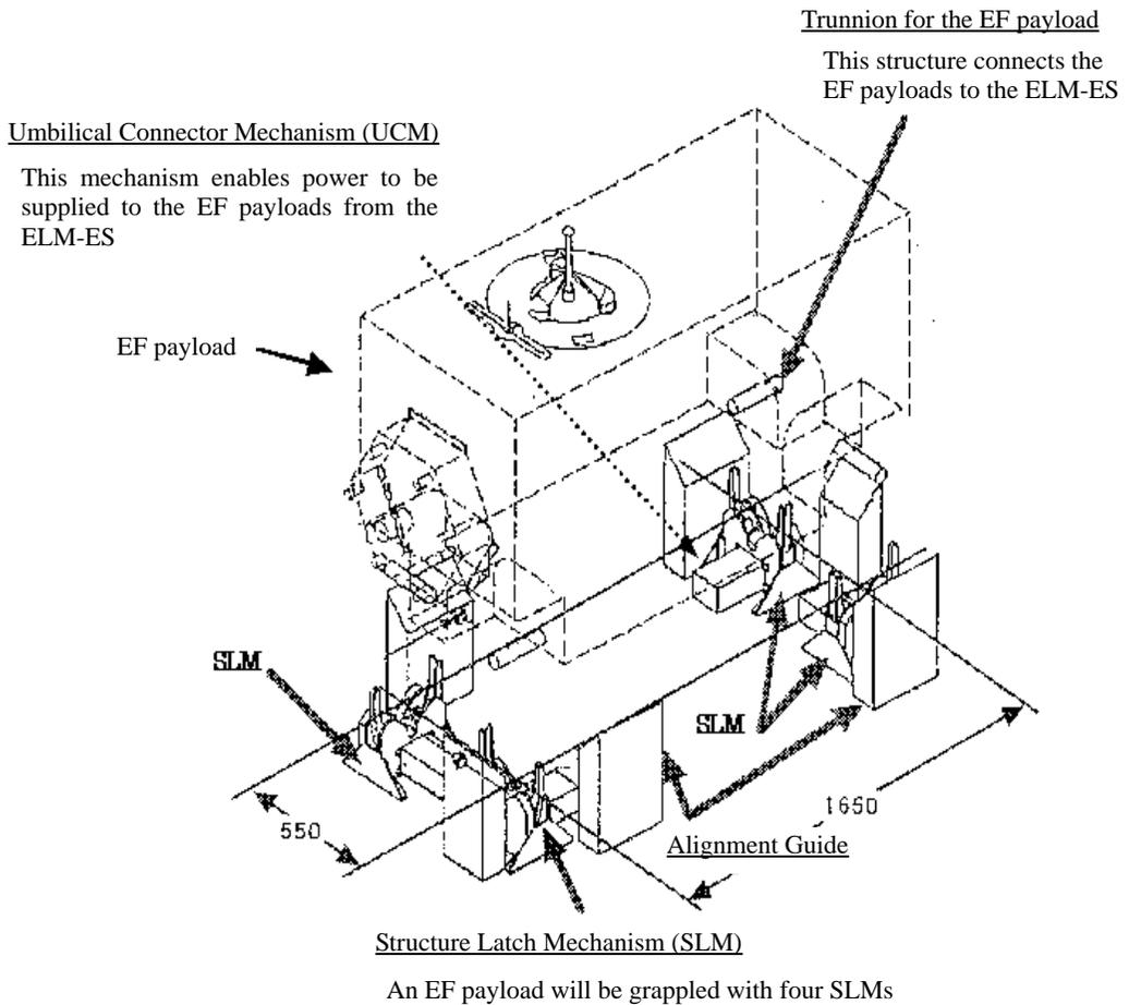
Figure 4.4.3-1 Payload Attachment Mechanism (PAM)
