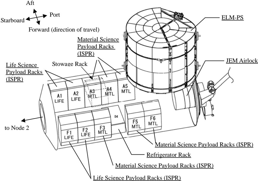
Figure 4.1.2-4 Experiment racks (ISPRs) inside PM
