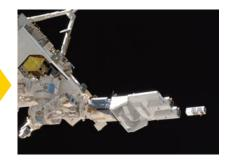
The robotic arm of "Kibo" holds the MPEP to transfer it to the release point. The satellites are deployed by a command signal sent from ground.
