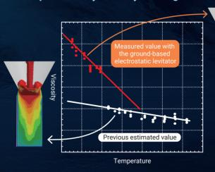
Comparison of the fluid simulation results for casting using the values of viscosity actually measured by experiments on Earth, using the ground-based electrostatic levitator with the previously estimated values. The accuracy of the simulation has been improved by using the measured physical property
