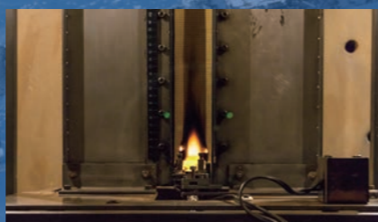
Material flammability evaluation test (NASA standard)
