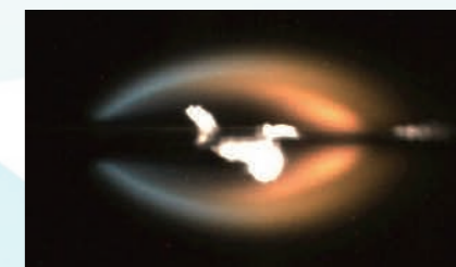
Image of flames spreading over a filter paper sample ©Hirosaki University/Gifu University/Hokkaido University/JAXA
