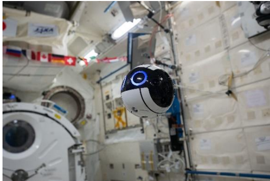
"Int-Ball" is a camera drone which can record video while moving in space under remote control from the ground.
